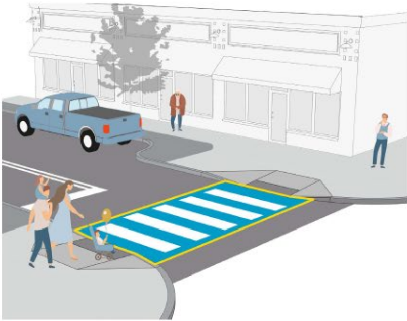
Upgraded high-visibility crosswalks: Improve visibility for people crossing the street.
